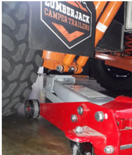
Vehicle Jack in position on trailer
