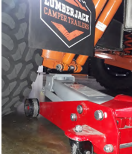
Vehicle Jack in position on trailer
